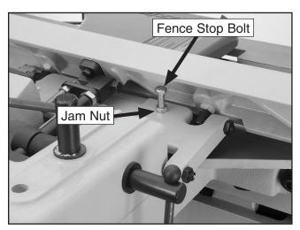
Figure 67. 45° outward fence stop jam nut.
